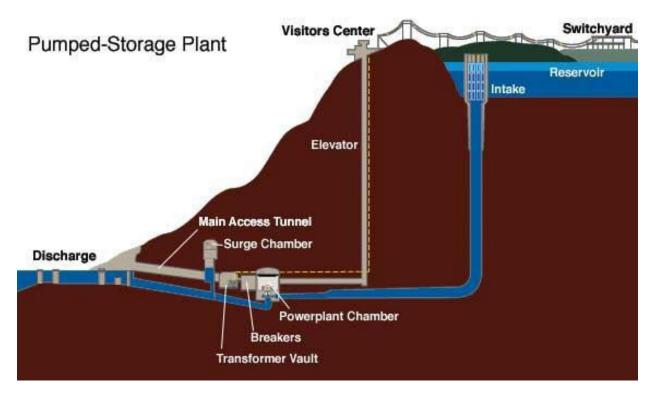
Figure : A basic schematic of the pumped hydro installation at Raccoon Mountain
