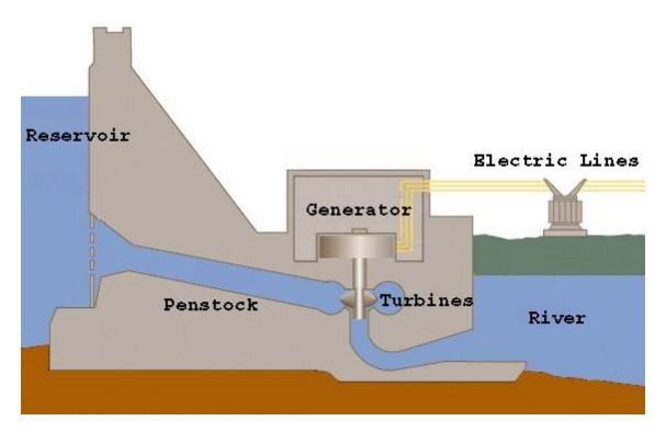
Figure : Diagram of a hydroelectric facility
